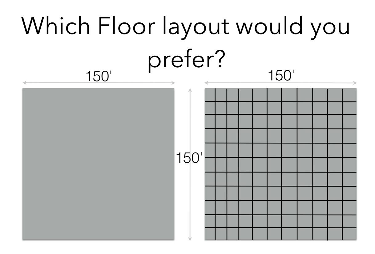
Conventional concrete requires countless linear feet of contraction (control) joints
