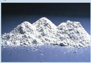
Fig. 1. White cement is subject to exacting quality control procedures that minimize color variation during manufacturing. This provides a neutral base for concrete finishes whether they are white or tinted.
