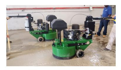
d) Polishing – All dry polishing and treatments were done with a high-speed burnisher and special burnishing pads. The materials used in the final treatment actually did more than spread a coating over the surface, however. The patented products integrated *into* the tiny surface capillaries, actually making them part of the surface itself. This bond produces a highly protective surface that out-performs traditional epoxy treatments at a fraction of the cost.
